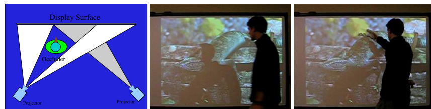
Fig. 4. Overhead diagram of a switching virtual rear projection system (left). As an occluder (the user) blocks one projector (center), the secondary projector begins to fill in the shadow (right). Footnote 3 provides a URL to download the video from which the center and right images were taken. The video illustrates the system's capabilities much better than static images.
