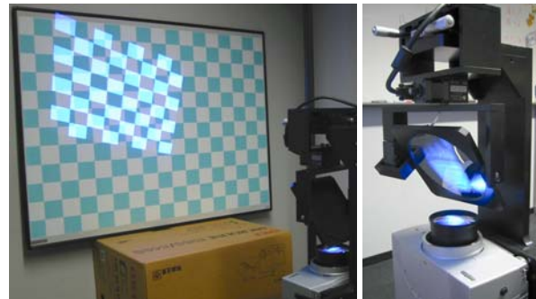
Figure 1. Steerable projector incorporating a pan-tilt mirror displaying a calibration pattern on a checkered surface.
