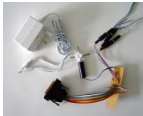
Figure 21 The buttons on the crayons are connected to the computer's serial port via a special piece of hardware
