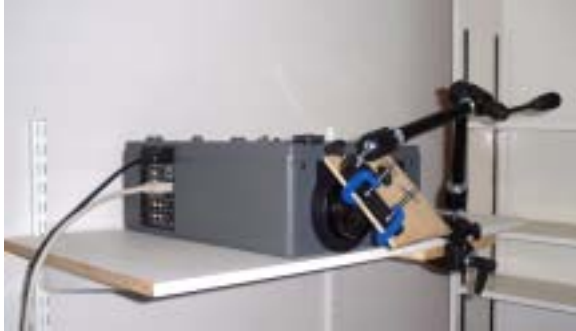
Figure 26 Projector on a shelf with image its reflected downward
