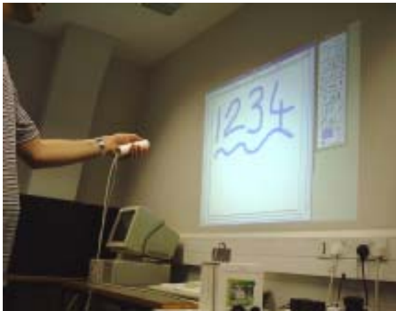
Figure 24 An unmodified X Windows drawing program controlled by pointing a crayon at the wall
