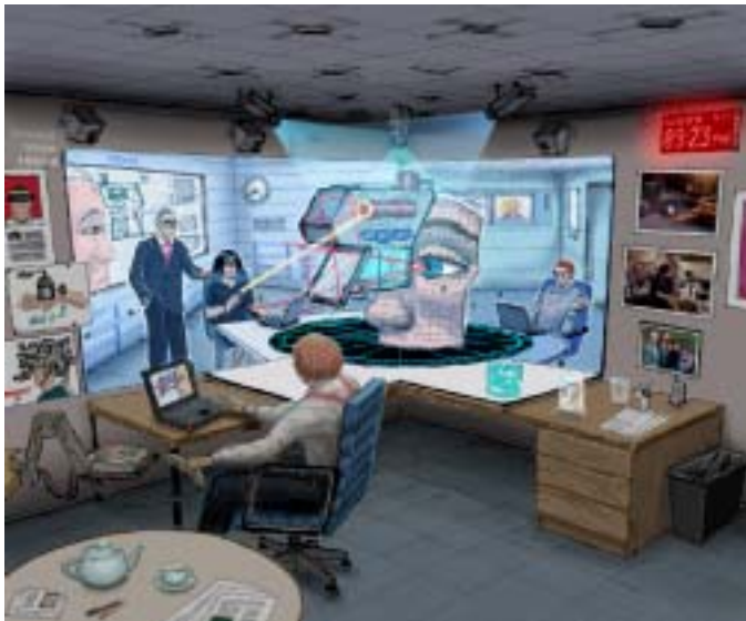
Figure 10 A sketch of the Office of the Future [44]. Multiple cameras infer the geometry and reflectance of the visible surfaces and multiple projectors project images onto them.
