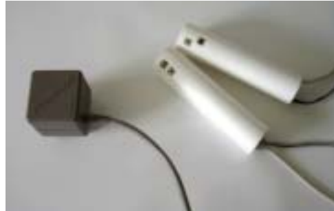
Figure 20 The magnetic transmitter (left) produces a field that is detected by the receivers in the crayons (right)
