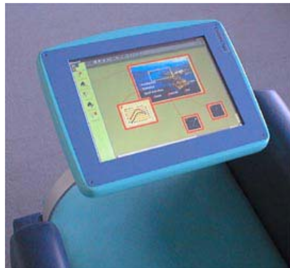
Figure 18 The CommChair with integrated pen-based computer [54]
