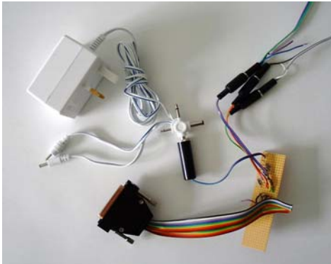
Figure 3: The buttons on the crayons are connected to the computer's serial port via a special piece of hardware
