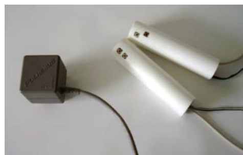
Figure 2: The magnetic transmitter (left) produces a field that is detected by the receivers in the crayons (right)
