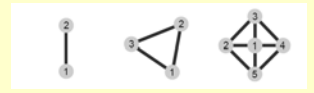
The projector-to-surface homographies are not independent. The graphs above show the constraints between them, where the nodes are homographies and the edges are the constraints.
