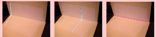
Lines are displayed by the projector. Kinks in the projected lines indicate the location of the boundary between the surfaces
