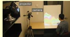
A user at a two-surface projected interface. The projector and camera can be mounted at the side.
